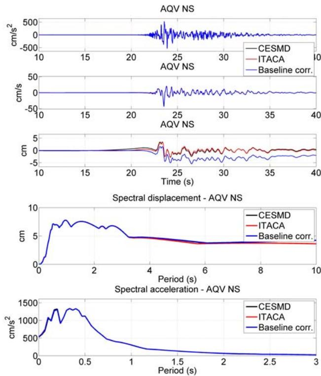
Figure 4. As Fig. 2, for the AQV corrected record, NS component, from the  $M_w$ 6.3 L'Aquila earthquake, 2009. Superimposed is the record corrected with a piecewise baseline on velocity to retrieve permanent displacements.
