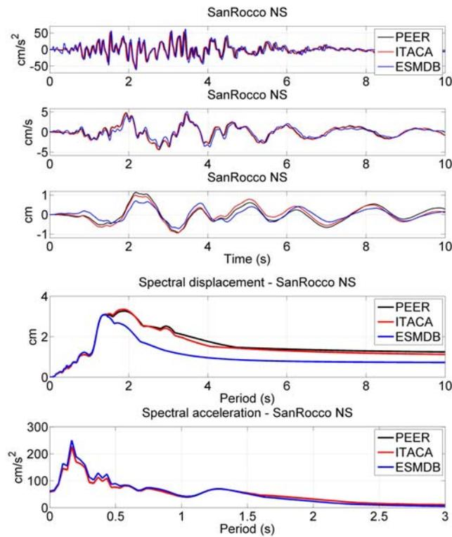
Figure 2. Comparison of San Rocco corrected record, NS component, from the  $M_w$ 6.1 Friuli aftershock of Sep 15 1976, 03:15 GMT, as available from ITACA, ESMDB and PEER databases. From top to bottom: corrected acceleration, velocity, displacement, spectral displacement and spectral acceleration.
