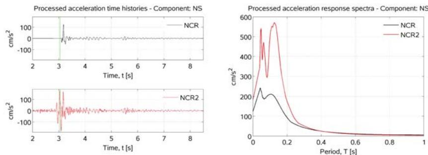
Figure 6. Analogue (NCR) and digital (NCR2) corrected accelerograms of event 19971014\_075405 (NS component in Table 1).
