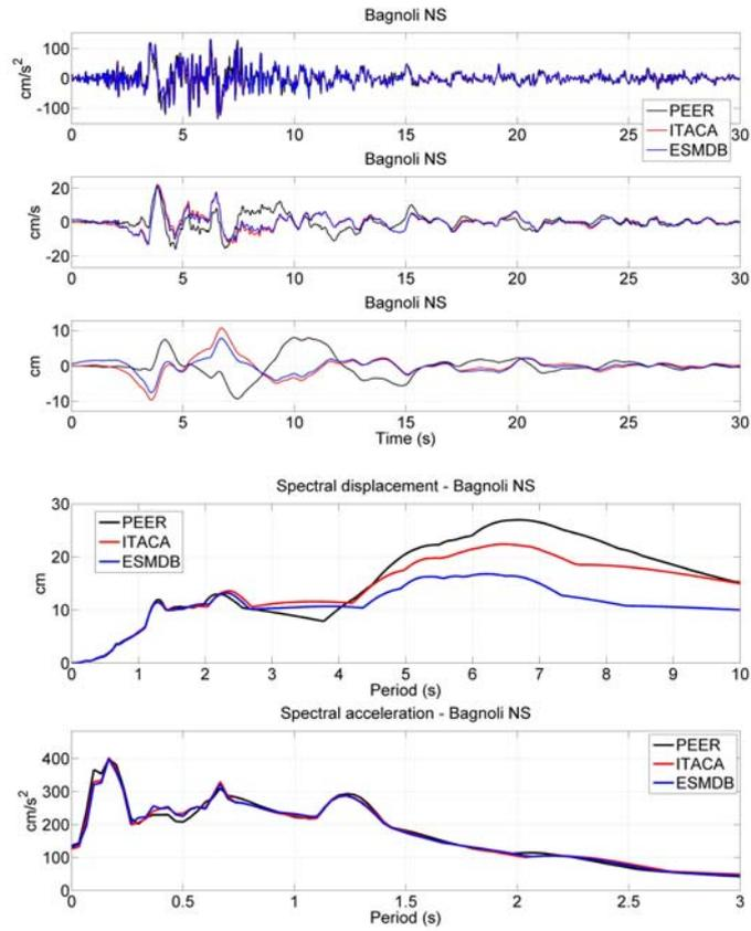
Figure 3. As Fig. 2, for the NS component of Bagnoli corrected record, from the  $M_w$ 6.9 Irpinia earthquake, 1980.
