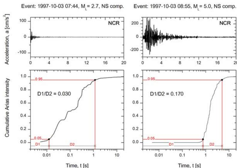
Figure 5. Two analogue records from the same station NCR, identified as *late triggered* (LT, left) and *normally triggered* (NT, right).
