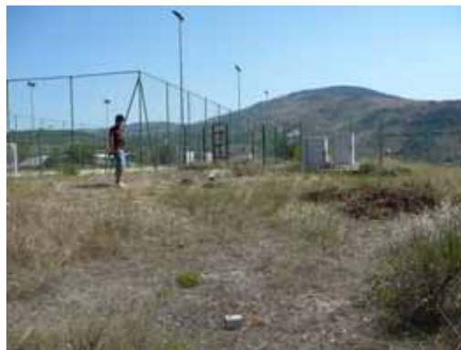
Figure 11. HAVSR measurements at the CPS RAN station. The silver small object at the bottom of the picture in the tromograph Tromino used for single station ambient vibration measurements.
