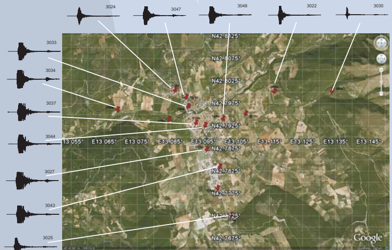
Figure 7: Temporary seismic array in Norcia. The recordings of the 6 April 2009 mainshock of the L'Aquila sequence and of an aftershock are shown. Note the variability of ground motion within the basin, also clear in the clipped recordings of the mainshock.
