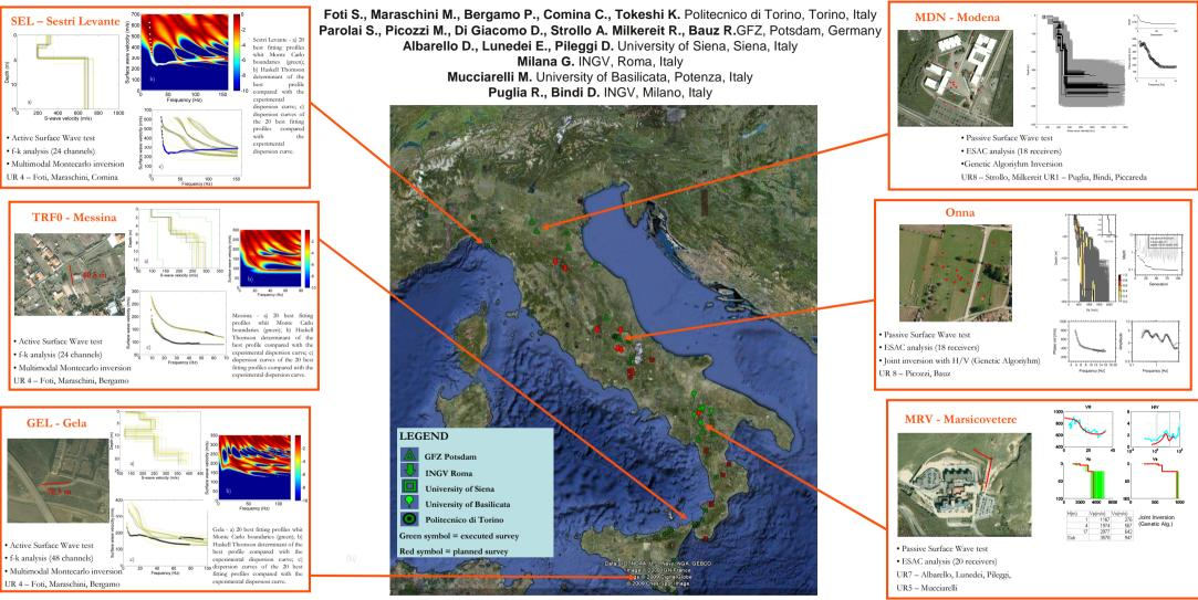
Task 3 of project S4 is devoted to improve the knowledge of the sites of the Italian Accelerometric Network (RAN), mainly by providing a reference shear wave velocity profile for each station. Surface wave tests have been selected as the primary tool for the characterization, due to their flexibility and cost effectiveness. We report on the ongoing activities and we show some of the already available S-wave velocity profiles.
