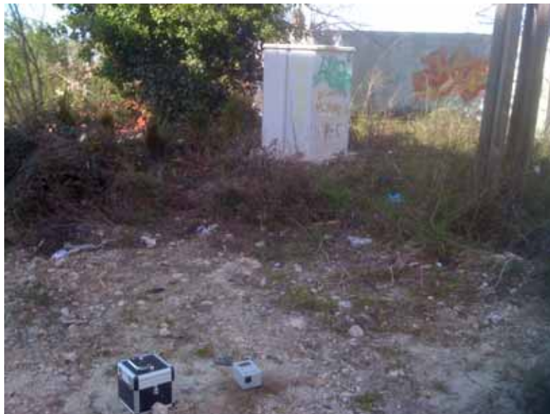
Figure 5. Location of the Vibo Valentia RAN station. On the bottom, the digital tomograph used for the single station ambient vibration measurements is shown
