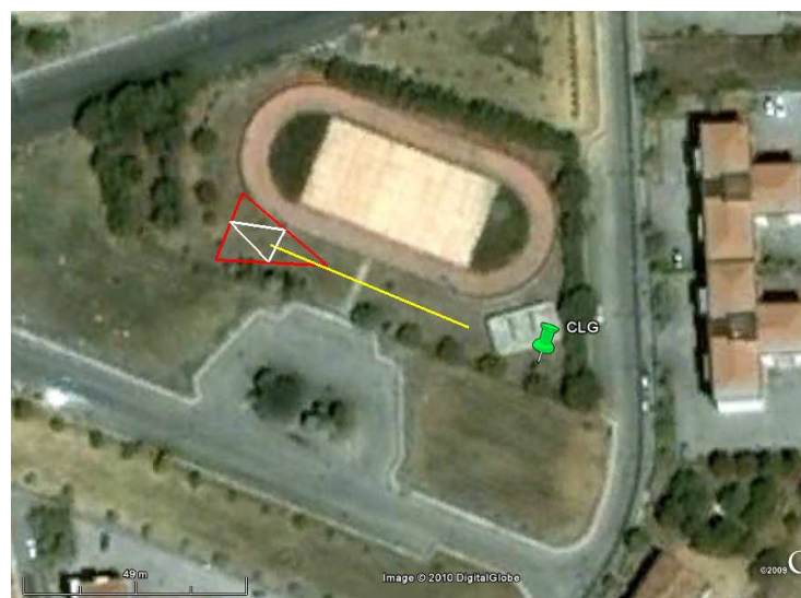
Figure 2 Caltagirone: array map. The yellow line represents the active measurements array; the red triangle and the white triangle represent the two triangles along which receivers for passive measurements were arranged.
