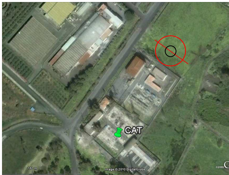
Figure 2 Catania (Piana): array map. The red line represents the active measurements array; the black circle and the red circle represent the two circles along which receivers for passive measurements were arranged.
