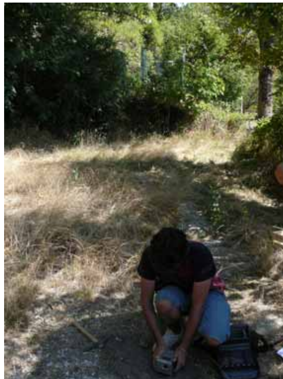
Figure 5. Location of the Scanno RAN station (in the background). On the bottom, the digital tromograph used for the single station ambient vibration measurements is shown
