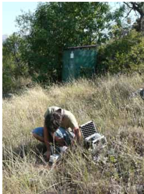
Figure 5. Location of the L'Aquila – Colle dei Grilli RAN station (in the background). On the bottom of the picture, the digital tromograph used for the single station ambient vibration measurements is shown
